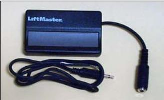
This transmitter has a 1/8" mini-phone jack on the side surface. Also includes a 1/8" mini phone plug with 30" of cable. This kit is used to allow activation by E.C.U. and custom switches. Momentary contact closure required for activation. Size 3" x 1.75" x 0.62".
