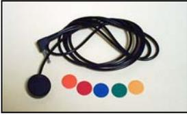
This is a sensitive switch for those people with very limited hand use. It has to be plugged into an E.C.U. transmitter (B) below.
