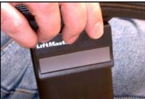
This transmitter may be mounted below the wheelchair armrest or a side panel. Includes a 1/2" thick riser bar that can be mounted on the button to provide a long raised
